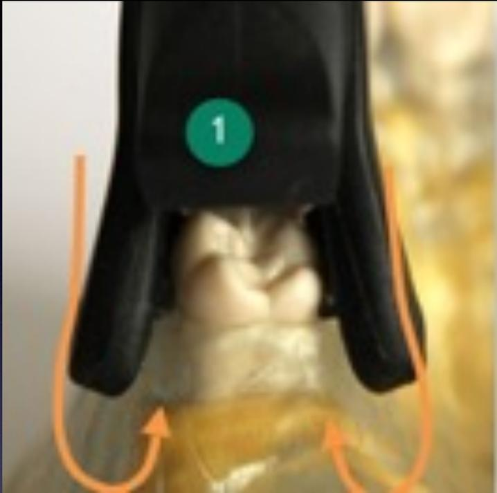
1-Flexible “arms” on end of tip straddle the tooth and Near-infrared photons are emitted through these arms
