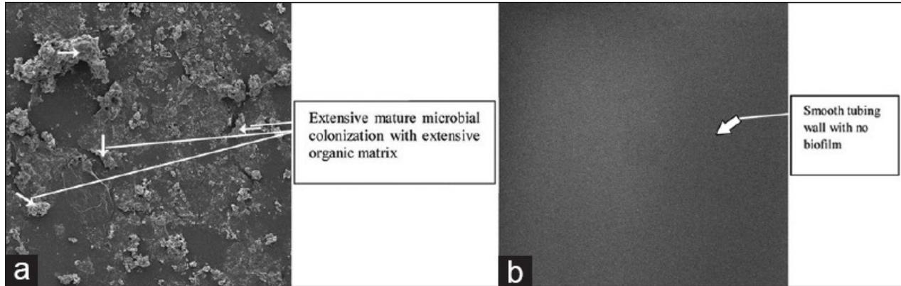
Scanning electron microscope images show the efficacy of the disinfectant or disinfection procedure. (a) The inner lumen wall of the cut section from the untreated dental waterlines (control tube) and the arrow indicates extensive mature microbial colonization with extensive organic matrix material. (b) The inner lumen of the cut section of treated dental unit waterline (sample a) and the arrow indicates the smooth tubing wall with no biofilms
